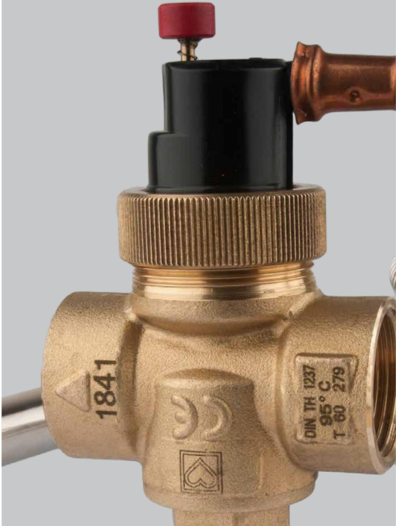
Thermal safety valve prevents excessive temperatures in boilers on solid fuel in water-based heating systems in accordance with EN 12828 norm.
